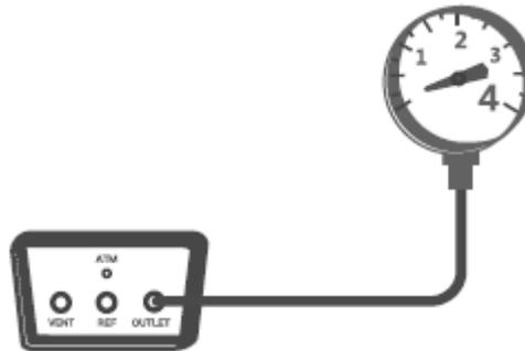
Figure 3- 12 Calibration of a pressure gauge
