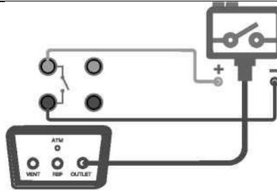
Figure 3- 16 Calibration of a pressure switch
