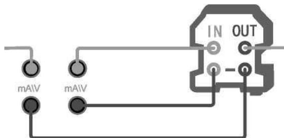
Figure 5- 3 Calibration of the signal isolator
