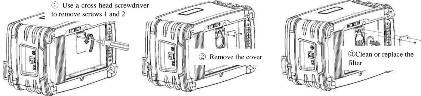
Figure 8- 1 Disassembly of the suction filter
