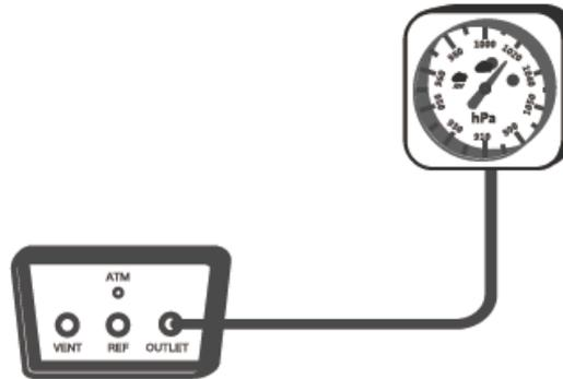
Figure 5- 9 Calibration of the aneroid barometer
