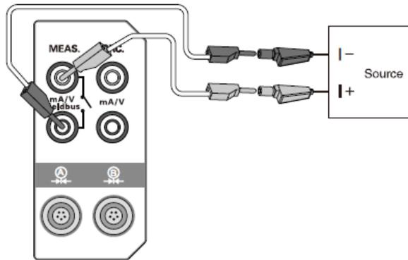
Figure 3- 5 Current measurement
