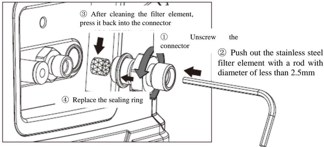
Figure 8- 3 Disassembly of differential pressure connector
