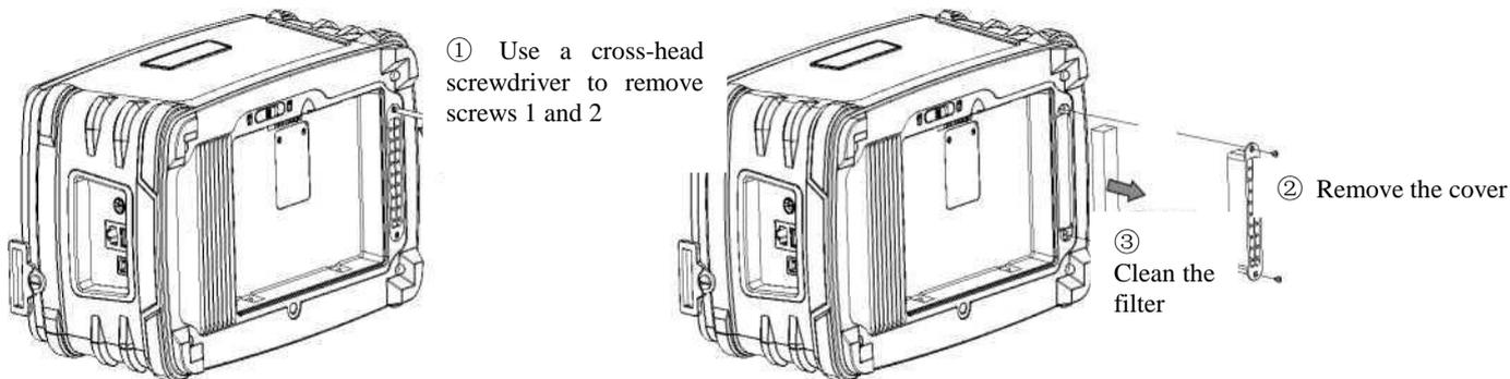
Figure 8- 4 Disassembly and assembly of the air filter
