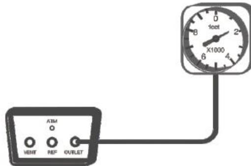
Figure 5- 10 Calibration of the barometric altimeter
