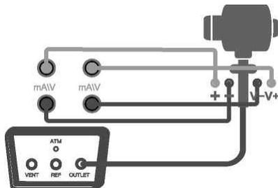
Figure 5- 2 Calibration of the pressure sensor
