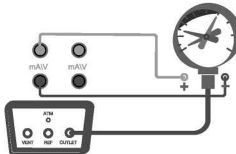
Figure 5- 4 Calibration of the contact pressure gauge
