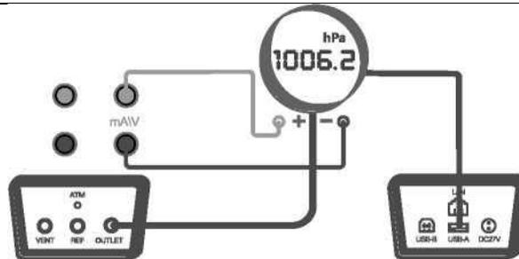
Figure 5- 7 Calibration of the VAISALA digital barometer
