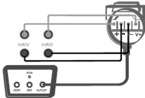
Figure 3- 15 Calibration of a 4-wire pressure transmitter
