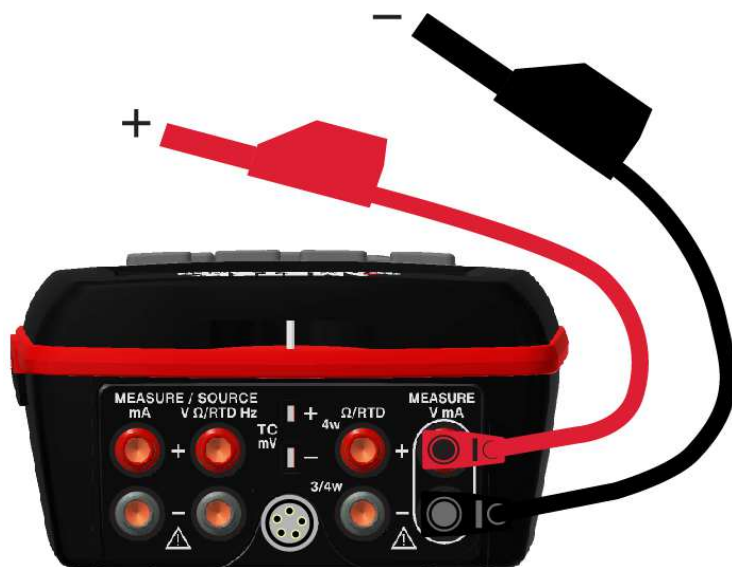
Figure 13 mA current measurement connection (upper window)
