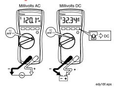
With the function switch in the  $\overline{m^{\widetilde{V}}}$  position, the Meter measures ac plus dc millivolts. Press \_\_\_\_\_ to switch the Meter to dc millivolts
