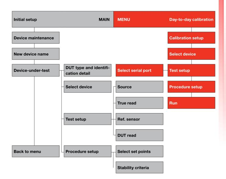
The unique "Icon bar" is key for easy set up of a calibration task. The "Icon bar" tells the current status of the calibration process, starting with selection of the sensor to be calibrated and ending with the performance of the calibration. The diagram shows the basic steps needed to set up a calibration.
