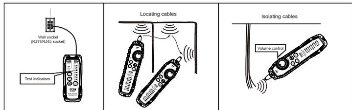
If the target cable are intermixed with massive cables, turn the sensitivity knob to adjust the sensitivity. Louder sound means stronger signal and closer to the target cable.
