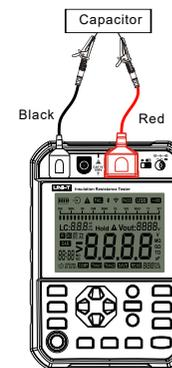
Fig. 9.3.3.1 Wire connection of capacitance measurement
