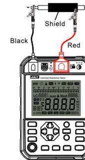
Fig. 10.1.1 Two-wire connection
