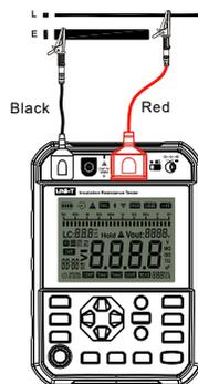
Fig. 9.3.2.1 Wire connection of voltage measurement
