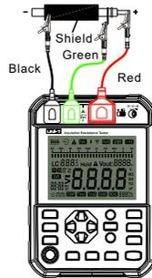
Fig. 10.1.2 Three-wire connection
