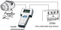
This application allows mA measure and source modes to be used through the Hart® communicator.
