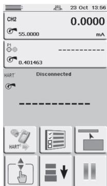
Turn on the internal HART<sup>®</sup> resistor. This can be selected by pressing
