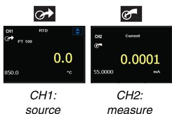
When first using the calibrator, there are default measure and source functions on the display:
