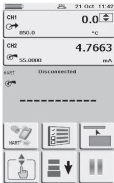
2. Set-up the HART<sup>®</sup> device, if loop power required, use CH2 for current (24V).
