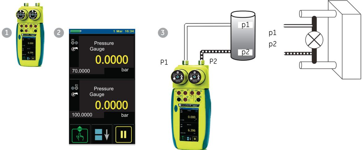
1. Assemble the pressure indicator with the correct PM 620-IS modules; see [Section 4.2.1](#).
