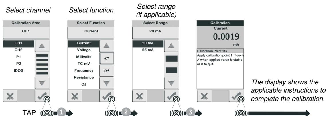
When the calibration is complete, set the next calibration date; see [Section 2.10.1 \(Advanced: Calibration options\)](#).
