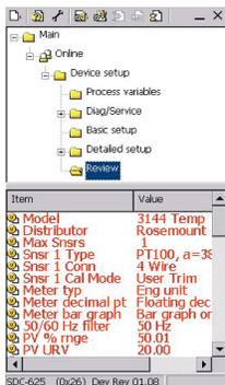
This is the ideal starting point for finding out information on the configuration of the HART<sup>®</sup> transmitter. It provides details of the model, distributor, tag, serial number, sensor & trim limits, alarm parameters, saturation limits, damping and span limits etc.
