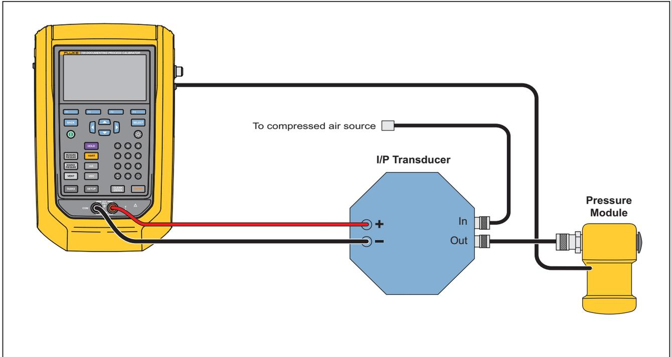
**Figure 13. Current to Pressure Test (I/P) with External Pressure Module**
