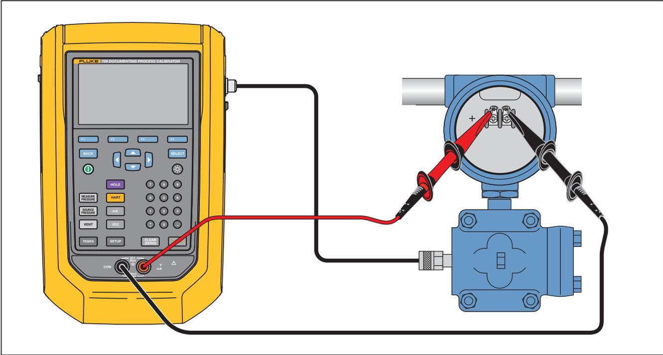
**Figure 11. Pressure Transmitter (P/I) Task Connections**
