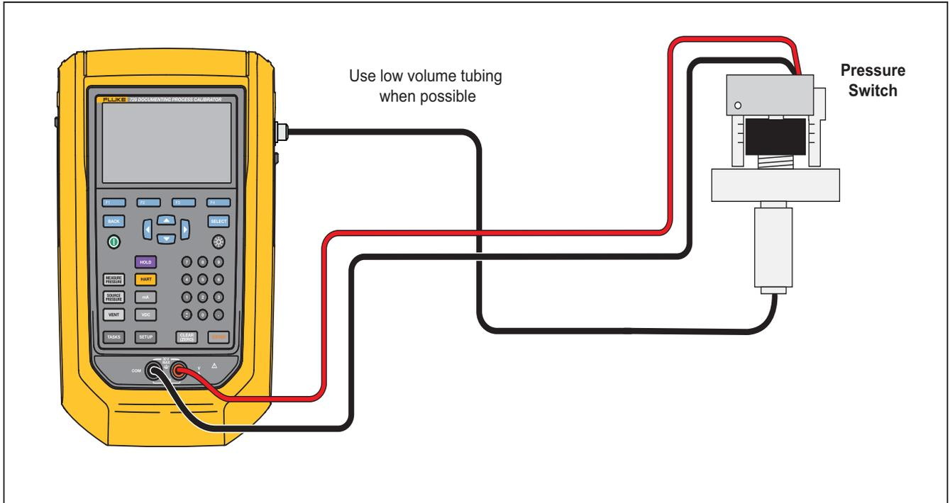
**Figure 12. Switch Test Connections**
