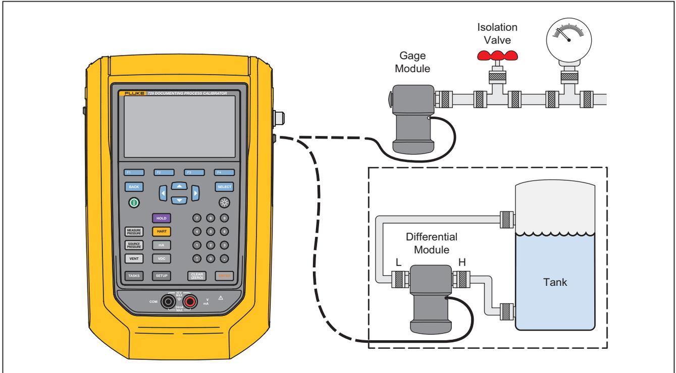
**Figure 19. Pressure Module Connections**
