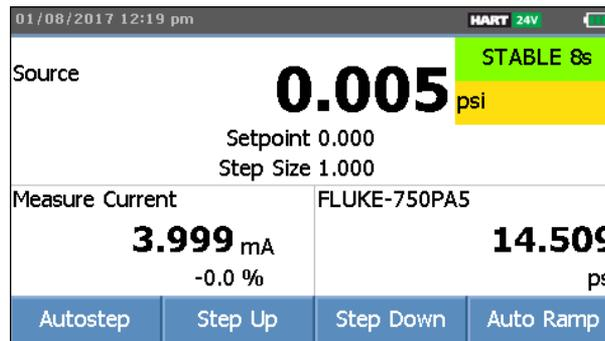
**Figure 6. Triple-Function Display with External Pressure Module Connected**
