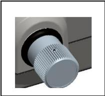
When pressurising large volumes this can be used to refill the pump without releasing pressure from the UUT (see Section 0)
