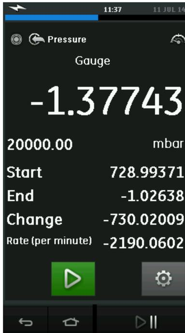
Figure 2-27 Leak Test Example
