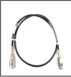
A high pressure pneumatic hose rated to 400 bar (5800 psi). The hose connects directly to the DPI612 pressure port and replicates the quick fit connection for compatibility with the standard adaptors supplied and the other adaptor kits.
