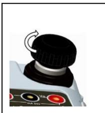
Open the pressure release valve counter clockwise (1 turn)
