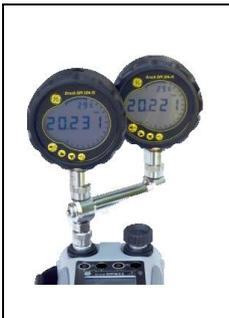
For greater efficiency, two test devices can be connected at the same time. The adaptor connects to the pressure port of the DPI612 and provides two outlet ports. It is compatible with the standard adaptors supplied and the adaptor kits.
