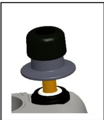
This control is used to fill and generate a priming pressure on the UUT (approx. 10 bar max)
