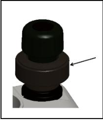
When pressurising large volumes this can be used to refill the pump without releasing pressure from the UUT (see Section 2.2.2)
