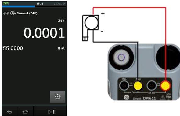
Figure 2-20 Measure current on CH1. Range  $\pm 55$  mA
