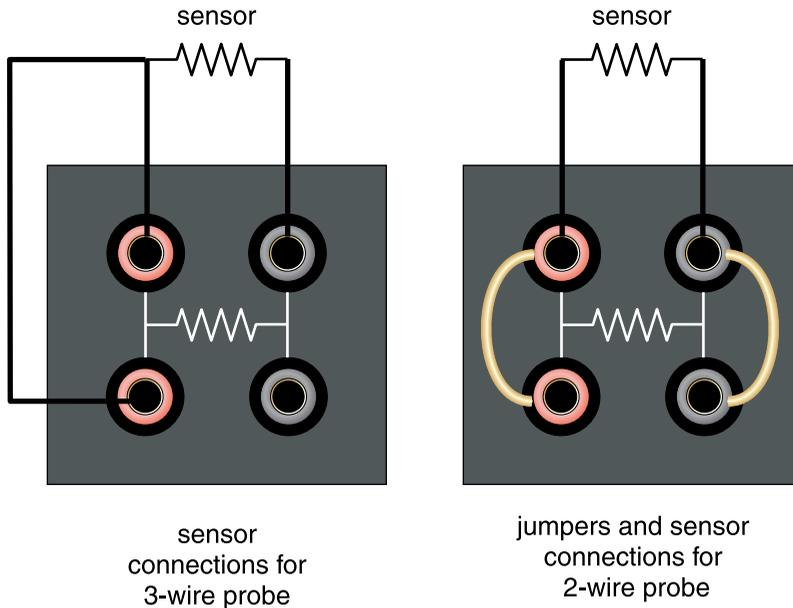
Figure 9 Jumper locations for 3-wire and 2-wire connections
