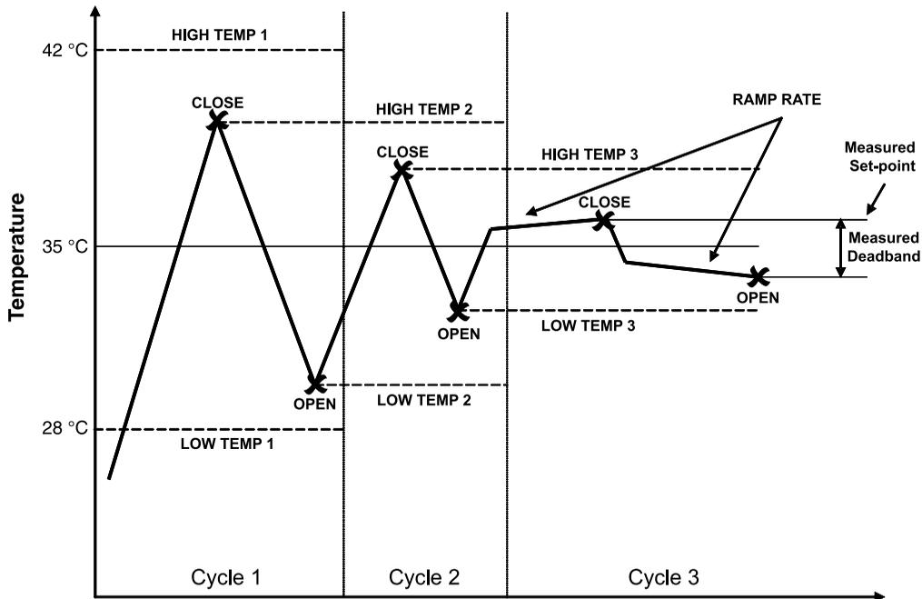
Figure 13 Auto and manual switch test operation example
