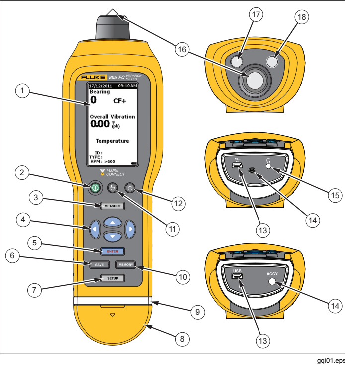
Figure 1. Meter Controls and Connections
