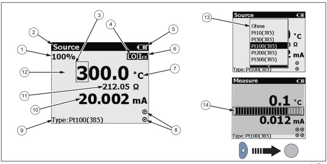
Figure 4. Elements of a Typical Display
