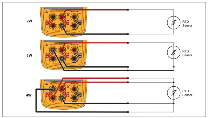
Figure 7. Measure Temperature with an RTD
