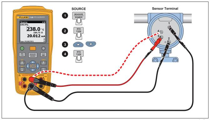
Figure 9. Connections for Simulating 3- and 4-Wire RTD
