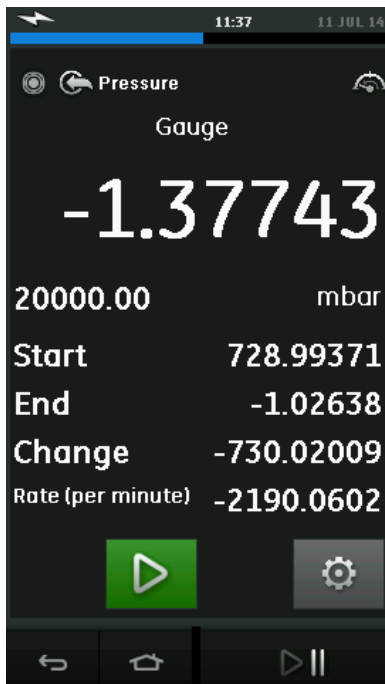
Figure 2-25 Leak Test Example
