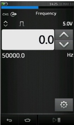
Figure 2-21 Example B - Source Frequency CH1 (Range 0 to 50 kHz)
