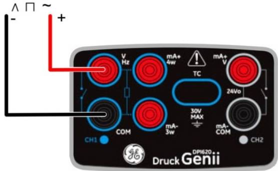
Figure 2-20 Example A - Measure Frequency on CH1 (Range 0 to 50 kHz)
