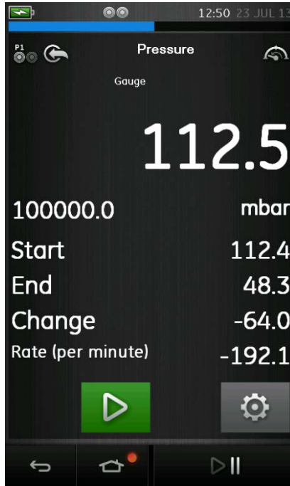
Figure 3-9 Leak Test Example
