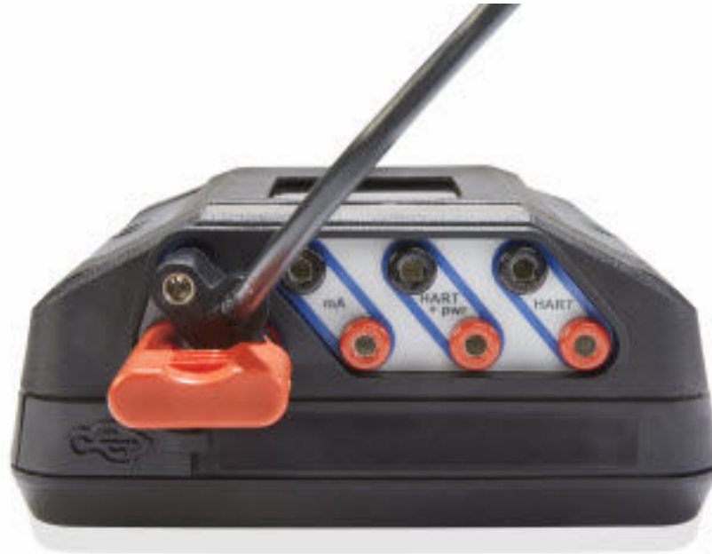
Figure 2-11: FOUNDATION fieldbus Power Plug attached to the Trex unit
