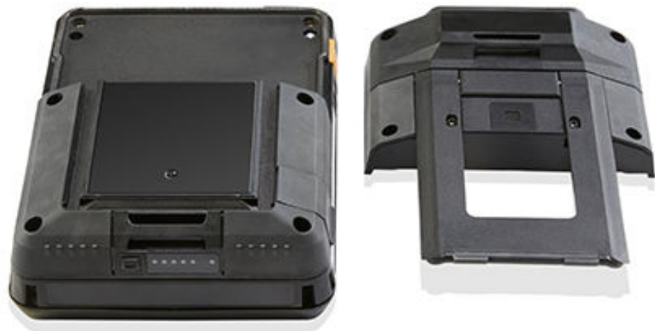
Figure 2-7: Trex unit with the communication module removed
