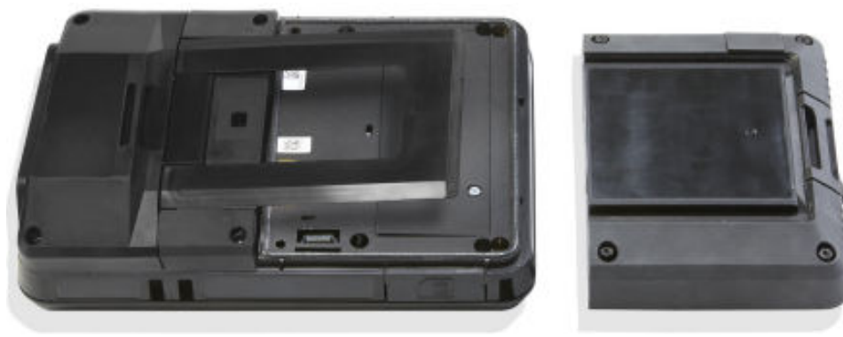
Figure 2-9: Trex unit with the power module removed
